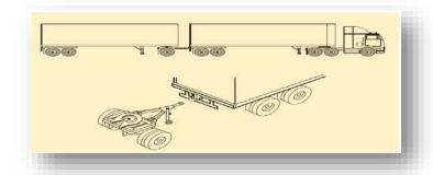
A train- example of a unit connected by a type A converter dolly
