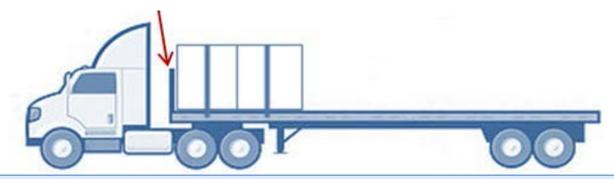
It is important to note that a cab shield is not a front-end structure or part of the cargo system
