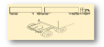
B train - example of a unit connected by a type B converter dolly.
