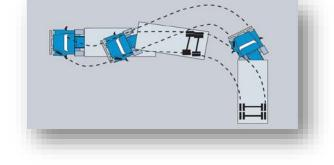
check for obstacles, possible hazards and clearance. After re-boarding, check mirrors and put the gear in reverse. Always select the lowest reverse gear available. Release park brake, start reversing, turning the steering wheel to the right to move the trailer to the left. Once the trailer is curving towards the space, turn the steering wheel to the left and let the tractor follow the trailer into the space.
