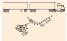
A train – example of a unit connected by a type A converter dolly.
