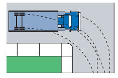
Be aware that, for every turn of the steering wheel, the rear wheels will follow a shorter path than the front wheels. Allow for this low speed off-tracking on every turn. Otherwise, your vehicle could hit another vehicle, or stationary object, or run over a curb and hit a pedestrian.
