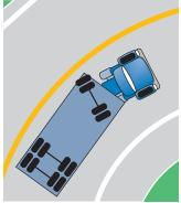
Keep the front of the vehicle closer to the centre of the road so the trailer wheels do not roll over the curb or drop off the pavement on the right.
