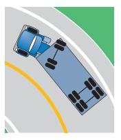
Keep the front of the vehicle closer to the outside of the curve (right side of road) so the trailer wheels do not cut into the other lane of traffic on the left.
