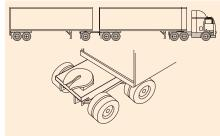
B train – example of a unit connected by a type B converter dolly.
