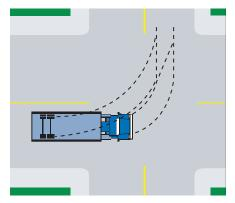
When turning left, ensure your vehicle's turning arc is wide enough to allow the vehicle to off-track on the left side without crossing the centre line. Your turn must be wide enough to prevent the vehicle from cutting the corner and hitting another vehicle. Complete the turn by driving to the right side of the centre line of the road entered.
