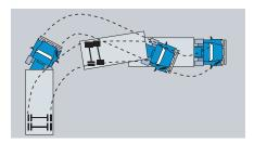
Reversing from the blind side uses the same steps as clear side reversing. However, it is harder to see where you are going. Once the reversing has started, you will mostly be using the right side mirror, including the convex mirror.
