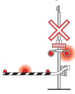
A controlled crossing is one with a flag person, stop sign, crossing gate or an electric or mechanical signalling device. All vehicles are required to stop at controlled railway crossings if signalled to do so.
