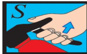
*Squeeze the handle slowly and evenly. Continue to squeeze until the fire is out and/or the fire extinguisher is empty.*
